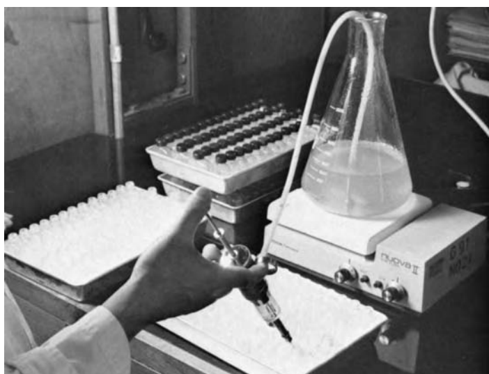
FIGURE 10.1 Filling the flat-sided bottles with medium.
